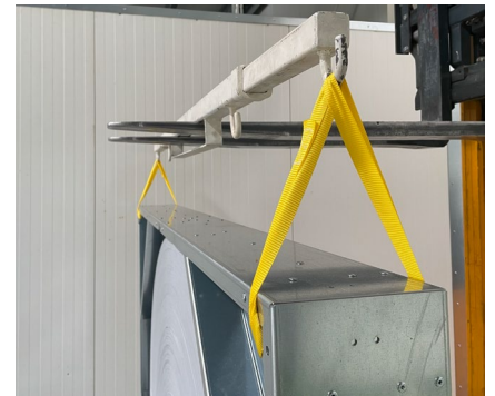
Figure 9 - SFC ERW lifting
