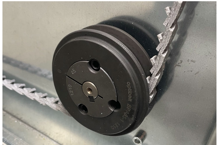
Figure 22 - Belt arrangement on the wheel and pulley
