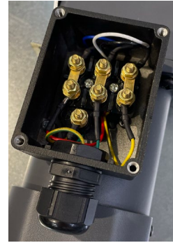
Default configuration of the junction box
